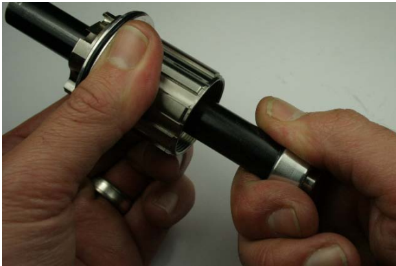
Fig.13 Pull axle out of freehub body.
