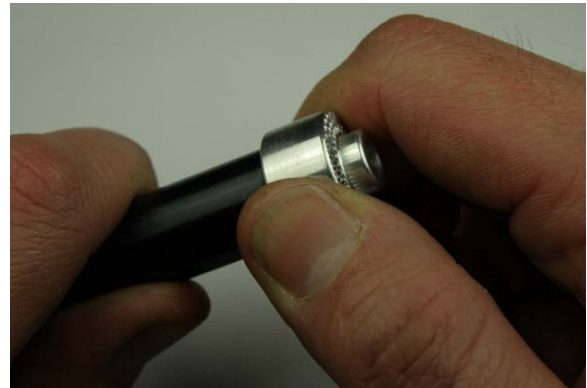
Fig.14 Checking fit of pressed on axle end.
