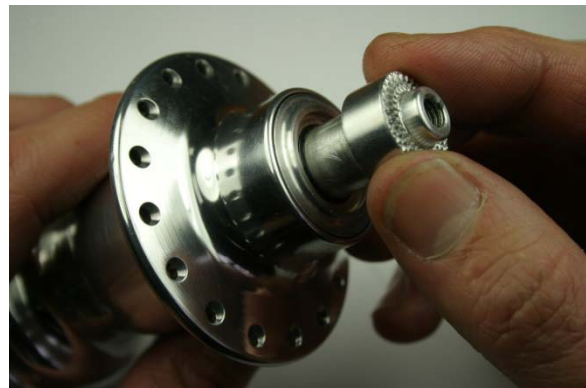
Fig.22 Inserting adjustable axle end.
