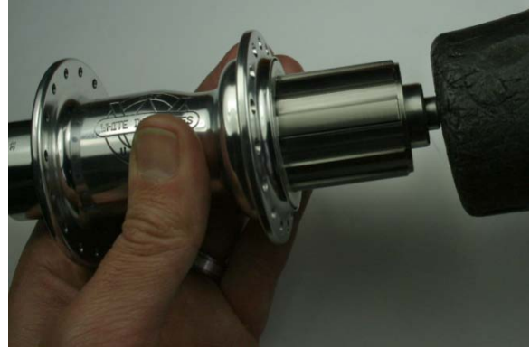
Fig.20 Tap axle end with mallet.
