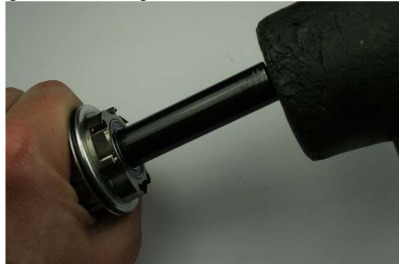
Fig.12 Tap axle through freehub body.
