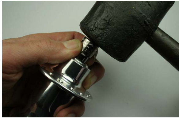
Fig.6 Tap socket to drive axle through shell.
