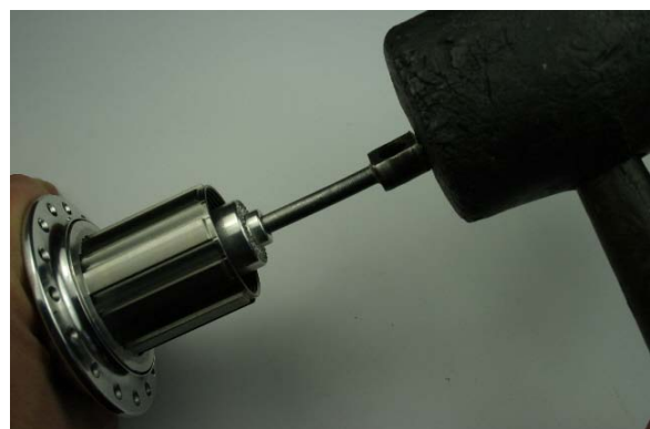
Fig.4 Tapping QR to free axle end.
