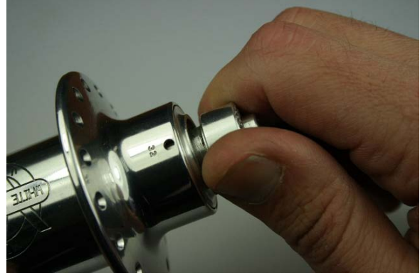
Fig.2 Remove axle end.
