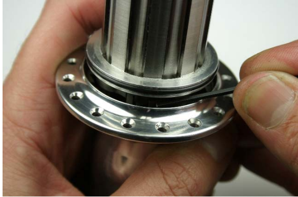
Fig.19 Freeing pawls with 2mm hex wrench.
