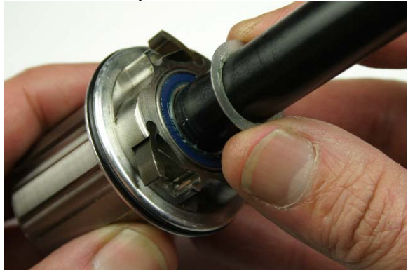
Fig.11 Remove thrust washer.
