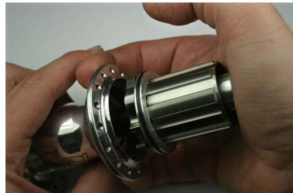
Fig.18 Slide axle through hub shell.
