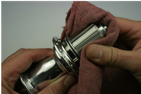
Fig.7 Pulling freehub body and axle out.
