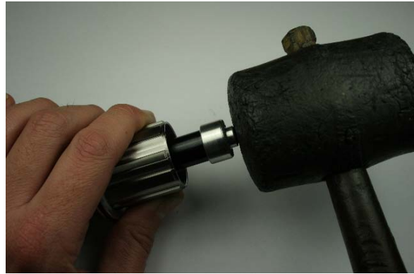
Fig.16 Tapping axle into place.
