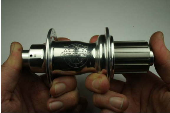
Fig.25 Checking hub for play.
