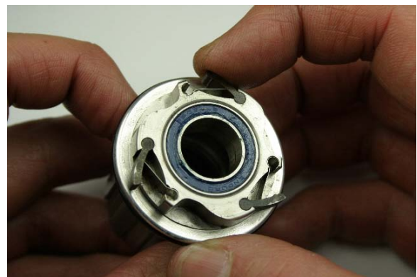
Fig.10 Checking pawl movement.
